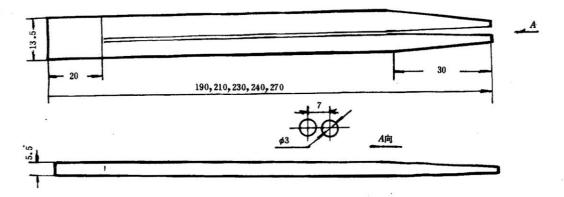
Figure 1. Diagram showing standard dimensions of bamboo chopsticks
